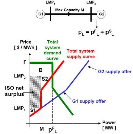
Fig. 2. Illustration of ISO net surplus collection for a simple 2-bus system with a branch limit  $M$  restricting power flow from the cheaper GenCo G1 at bus 1 to the load at bus 2. (Figure adapted from [11])
