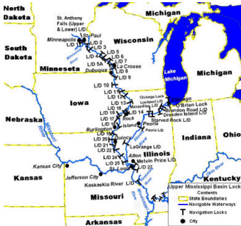
Figure 4.2.1. Locks on Mississippi and Illinois Rivers (source: U.S. Army Corps of Engineers website)
