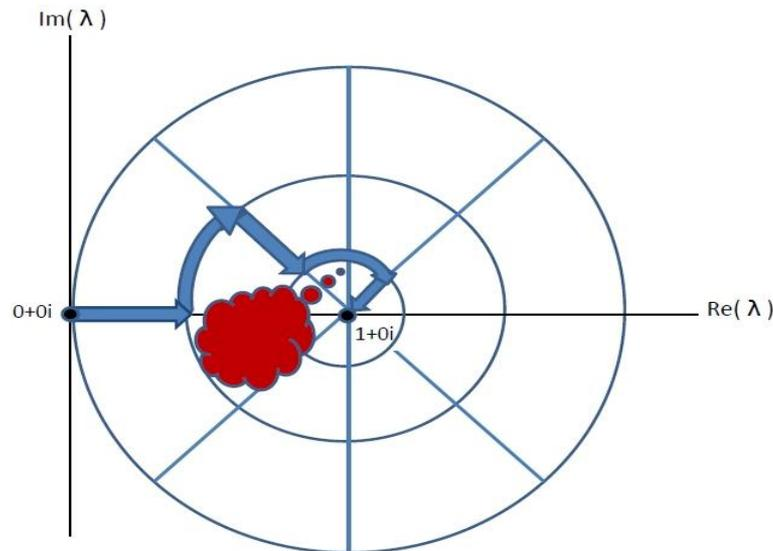
Adaptive movement of the homotopy continuation parameter  $\lambda$  from  $0+0i$  to  $1+0i$  in the complex plane, avoiding regions where computation becomes ill-conditioned
